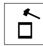
Protection against impact. IK 06 - 1,00 joule (version with frame) IK 08 - 5,00 joule (version with cover)
