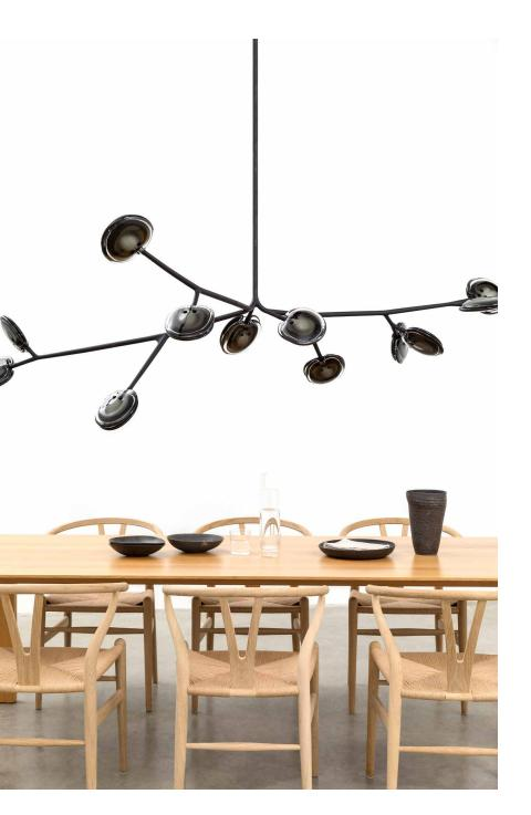
16 is formed by sequentially pouring three separate puddles of molten glass of varying opacity and colour over a horizontal plane. Each layer responds to the indeterminate shape of the previous pour to create a layered whole. Two of these pieces are then attached to house an internal light source.
