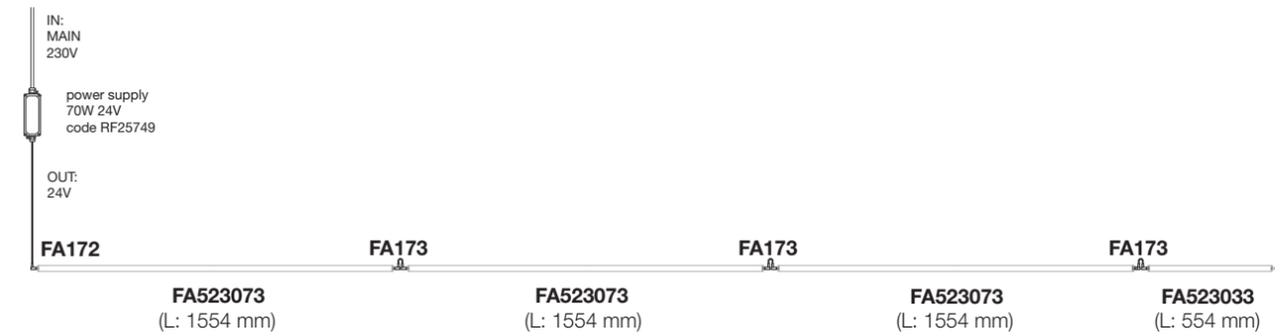
Maximale Länge 5 m / Max length in continuous 5mt
