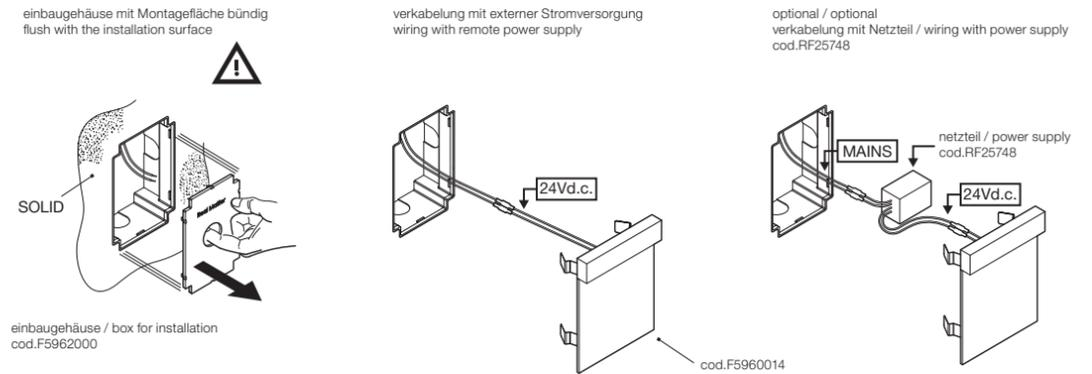
Einbau in Gipskartonplattenwand / Installation in Plasterboard Wall
