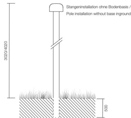
Stangeninstallation ohne Bodenbasis / Pole installation without base inground
