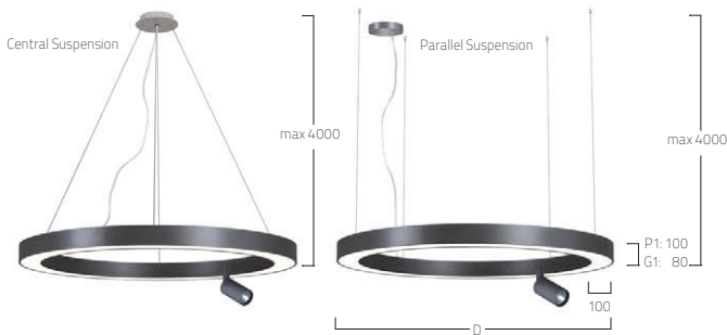
Minimal suspension height for the central suspension
