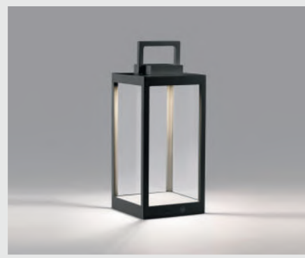
LANTERN T2 / Black / ART. No 270441 Design: Marie Holsting 8W LED - Rechargeable - 100 — 240V IP54 for indoor & outdoor - CRI > 90 2700K - Dimmable Dimensions: 150 x 150 x 320 mm
