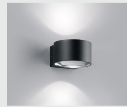
ORBIT W1 UP/DOWN / Black / ART. No 270581 Design: Nital Patel & Ronni Gol 2x8W LED - 230V - IP54 indoor & outdoor - CRI > 90 - 2700K - Dimmable Dimensions: 108 x 124 x 50 mm
