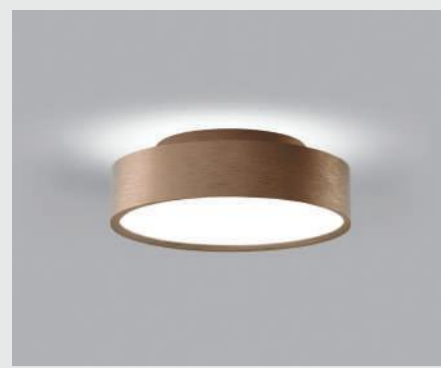
SHADOW 1 / Rose Gold / ART. No 270602 Design: Ronni Gol 7W+3W LED - 230V - IP54 indoor only CRI > 90 - 2700K - Dimmable Dimensions: Ø150 x 50 mm
