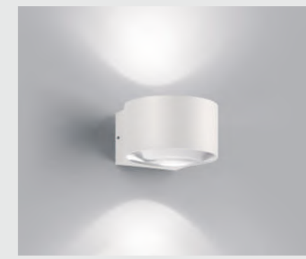
ORBIT W1 UP/DOWN / White / ART. No 270580 Design: Nital Patel & Ronni Gol 2x8W LED - 230V - IP54 indoor & outdoor CRI > 90 - 2700K - Dimmable Dimensions: 108 x 124 x 50 mm
