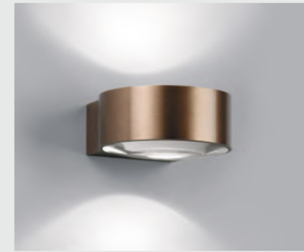
ORBIT W2 UP-DOWN / Rose Gold / ART. No 270592 Design: Nital Patel & Ronni Gol 2x12W LED - 230V - IP20 indoor only - CRI > 90 - 2700K - Dimmable Dimensions: 150 x 165 x 55 mm
