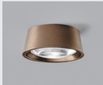
OPTIC OUT 1+ / Rose Gold / ART. No 270352 Design: Nital Patel AC10W LED - 230V - IP54 indoor only CRI > 90 - 2700K - Dimmable Also available in white & black* Dimensions: H: 50mm, Ø1: 110mm, Ø2: 130 mm
