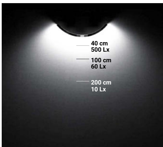
D-Wave + Rubber 3D Optics white 22W/m | 3000K
