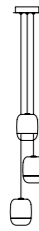
3R - 3S Ceiling Rose Ø 180 mm H 40 mm Cable 3000 mm Diffuser Ø 135 mm H 165 mm
