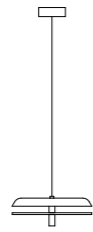
S3 Ceiling Rose Ø 120 mm Cable 3000 mm Diffuser Ø 350 mm H 130 mm
