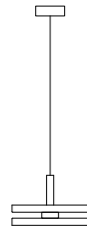
S3 Ceiling Rose Ø 120 mm Cable 3000 mm Diffuser Ø 330 mm H 210 mm
