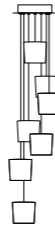
7R - 7S Ceiling Rose Ø 240 mm H 40 mm Cable 3000 mm Diffuser Ø 135 mm H 150 mm
