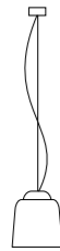
S1 Ceiling Rose Ø 80 mm Cable 2000 mm Diffuser Ø 240 mm H 265 mm
