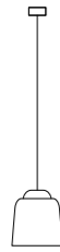
S1 Ceiling Rose Ø 80 mm Cable 3000 mm Diffuser Ø 240 mm H 265 mm
