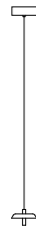
S1 Ceiling Rose Ø 120 mm H 40 mm Cable 3000 mm Diffuser Ø 120 mm H 76 mm
