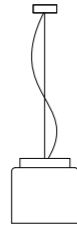
S5 Ceiling Rose Ø 120 mm Cable 3000 mm Diffuser Ø 360 mm H 350 mm
