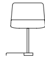
T1 H 430 mm Diffuser Ø 270 mm Base W 210 mm D 210 mm H 20 mm
