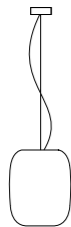
S5 Ceiling Rose Ø 120 mm Ceiling Rose LED Ø 160 mm Cable 2000 mm Diffuser Ø 360 mm H 450 mm
